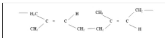
Since its molecular structure is close to that of natural rubber, which is a cis-isomer of poly isoprene, it has a number of similarities but a difference in form makes its mechanical properties
