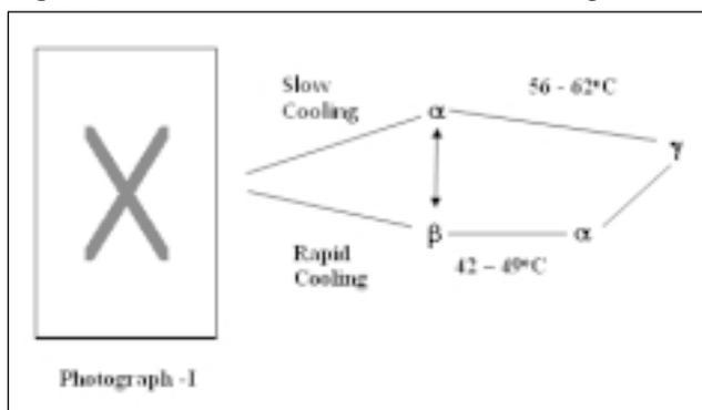
Materials expand, when heated from b to a or g phases (1-3%). When cooled down, shrinkage also takes place and it is greater than degree of expansion and differs by as much as 2%<sup>7</sup>.
